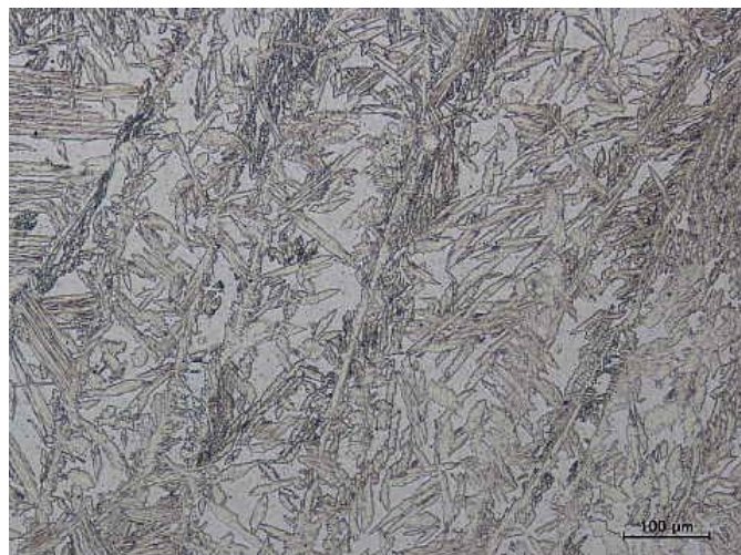
Fig.3 Microstructure of all-weld metal AA-2594
